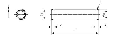
a Swaged chamfer at both ends.
